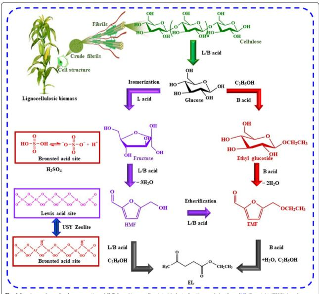
Fig. 1 Reaction pathway for the preparation of EMF from biomass. Reprinted (adapted) with permission from [12]. Copyright (2019) American Chemical Society
